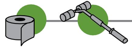
STEP 3: Install ZIP System™ flashing tape at the head of the window extending 1" past the jamb flashing tape. When a "T-Joint" occurs in the head of the window, ensure the vertical panel seam tape overlaps the head flashing. For alternative details please see page 30. Roll the Tape.
