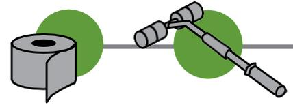
Install ZIP System™ flashing tape at all exterior corners with minimum 1-inch contact on overlay of both panels. For wider thicknesses, R-9 and R-12, use 6-inch ZIP System™ flashing tape or multiple pieces of 3-3/4-inch. Roll the tape once installed.
