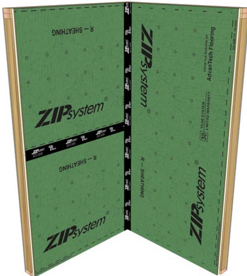
**PRO TIP:** Install ZIP System™ flashing tape in arm's lengths increments and work tape into corner with a plastic tool. For more tips see the technical tip, "*Proper Inside Corner Flashing with ZIP System Tape*"
