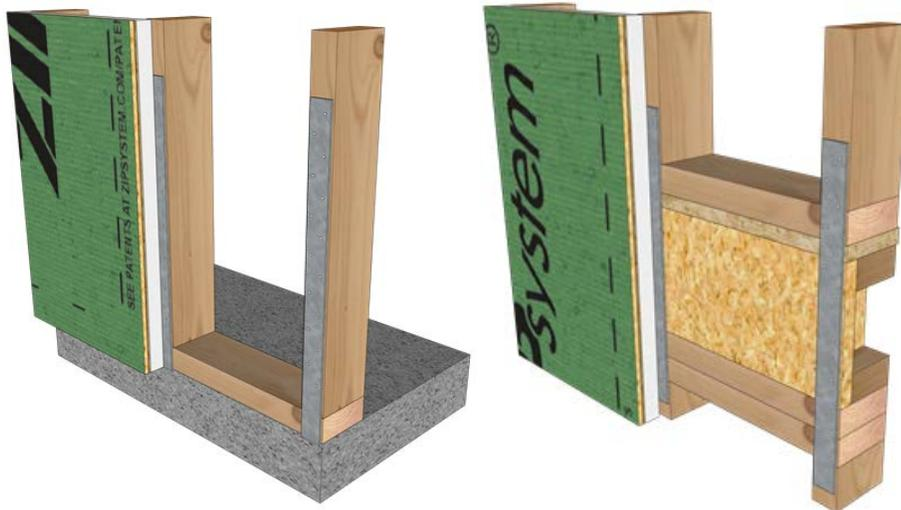
**PRO TIP:** Straps, ties and connectors installed on the exterior face of stud will not be visible after ZIP System® R-Sheathing panels are installed. Schedule any necessary anchor or nailing inspections accordingly.
