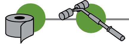
STEP 1: Tape the top edge of the weep screed flashing back to the ZIP System® R-sheathing. Install a mechanically fastened water resistive barrier equivalent to a Grade D felt paper after all ZIP System® R-sheathing panel seams have been taped. The building science industry promotes the use of a drainage gap behind porous claddings like stucco and adhered stone.
