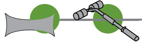
STEP 1: Install a piece of ZIP System™ stretch tape ensuring the tape extends a minimum of 6-inches up the jambs. Always follow window manufacturer's written instructions. Roll the Tape.
