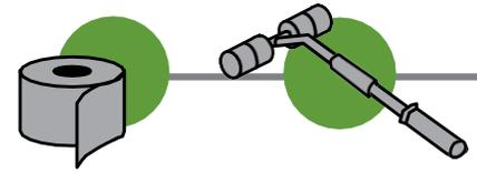
STEP 4: Install head flashing above window. Optional for self-flashed J-channel windows. Tape top of head flashing. From the back side of the window, install low expanding window/ door foam per the window manufacturer's installation guidelines. Roll the Tape.
