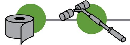
STEP 1: Tape the top edge of the masonry flashing back to the ZIP System® R-sheathing. Install brick ties in accordance with local building code and brick tie manufacturer's written instructions. Brick ties are to be installed into framing.
