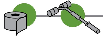
STEP 3: Install head flashing above door and then tape the top of heading flashing to the ZIP System® R-sheathing.
