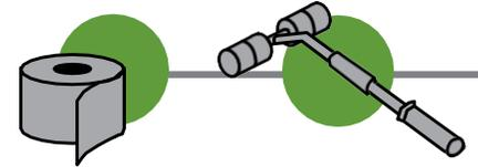
STEP 1: Tape top edge of drip edge back to the surface of ZIP System® R-sheathing. Install bottom wall flashing by other in accordance with designer of record or local building code.
