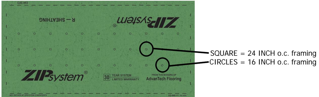
Install consecutive panels of ZIP System® R-sheathing with oversized foam sides of the panels in the same orientation to maintain proper spacing.
